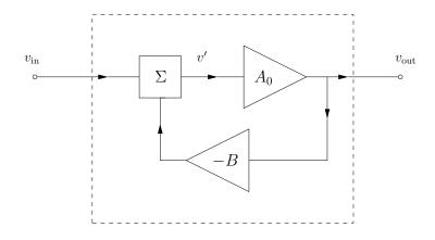
$$v_{\text{out}} = A_0 v' = A_0 (v_{\text{in}} - Bv_{\text{out}})$$
