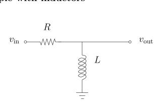
**Qualitative:** Consider this as a generalized voltage divider. Low frequency  $\implies$  low inductive impedance  $\implies$  small voltage across inductor  $\implies$  small gain. Conversely, high frequency  $\implies$  high inductive impedance  $\implies$  gain approaches unity. This is a high-pass filter.
