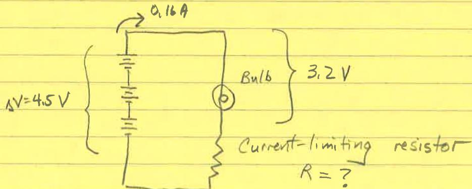
If we choose the right current limiting resistor to get  $I = 0.16 \text{ A}$ , the voltage drop across the resistor will be
