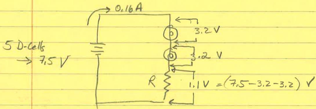
$$\text{In this case } R = \frac{1.1\text{ V}}{0.16\text{ A}} \approx 7\Omega$$
