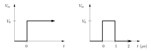
30. Sketch the approximate output from an RC differentiating circuit (i.e., an RC highpass filter) with  $R = 10 \text{ k}\Omega$  and C = 0.4 nF for the illustrated inputs. For the input on the left, make sure that your sketch of the output has an appropriate time scale indicated on the axis.
