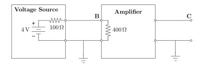
(c) When the amplifier is connected to the voltage source, and the load is connected across the output of the amplifier:
