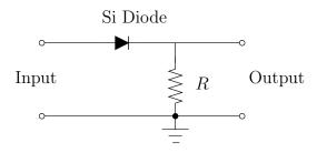
Sketch the voltage output waveform for each of the illustrated inputs.
