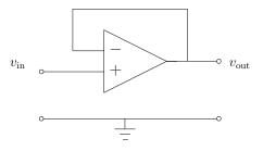
73. Sketch the output  $v_{\rm out}$  of the illustrated op-amp for the two illustrated inputs.
