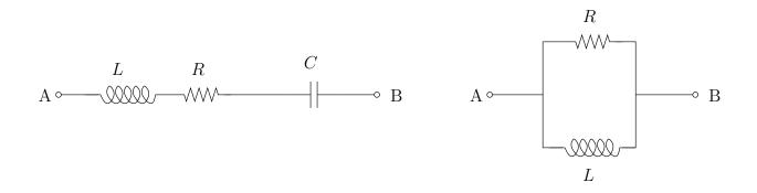
43. Calculate the impedance  $Z_{AB}$  in the form a + jb for the illustrated *RLC* combination.
