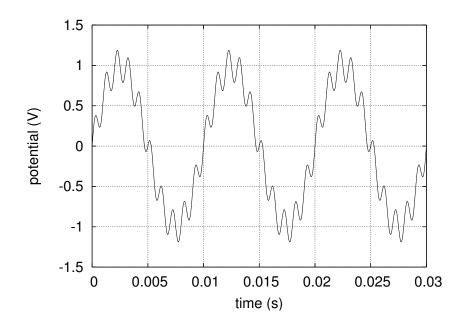
40. The illustrated voltage vs. time graph is a combination of a signal and unwanted 1000 Hz noise. Design a filter that will significantly attenuate the 1000 Hz noise, but leave the signal unattenuated.
