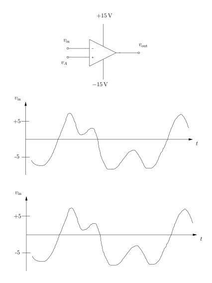
71. In lab you investigated the operation of a Schmitt trigger. Your trigger made transitions at reference voltages that were near 0 V. In the illustrated circuit the transitions have been shifted away from zero because of the voltage  $v_A$ . Determine the transition voltages for this more general Schmitt trigger. Express your answer in terms of  $v_A$ , R, and the saturation voltage of the op-amp  $V_{CC}$ . (You may assume that the negative saturation voltage is  $V_{EE} = -V_{CC}$ ).
