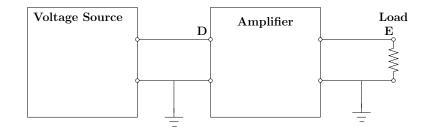
(d) Repeat the previous calculations for the loaded amplifier, except this time assume the the amplifier has an input impedance  $R_{\text{input}} = 10 \text{ k}\Omega$  and an output impedance  $R_{\text{output}} = 1 \Omega$ .
