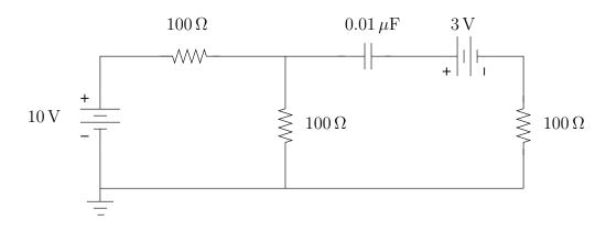
27. Consider the illustrated circuit that starts with the capacitor initially uncharged. The switch S is closed, and the capacitor begins to charge. What is the time interval between the time the capacitor is charged to 3 V and the time the capacitor is charged to 3.78 V?
