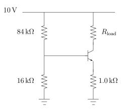
60. Consider the simple common-emitter amplifier discussed in class. (This is also part of the amplifier that some of you built in the optional part of the Introduction to Transistors Lab.) Consider as the input the voltage  $V_{\rm in} = 1.59 + 0.33 \cos(\omega t)$ , i.e., a signal that oscillates between 1.59 - 0.33 = 1.26 V and 1.59 + 0.33 = 1.92 V.
