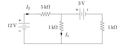
15. Calculate  $I_1$ ,  $I_2$ , and  $I_3$  in the illustrated circuit.
