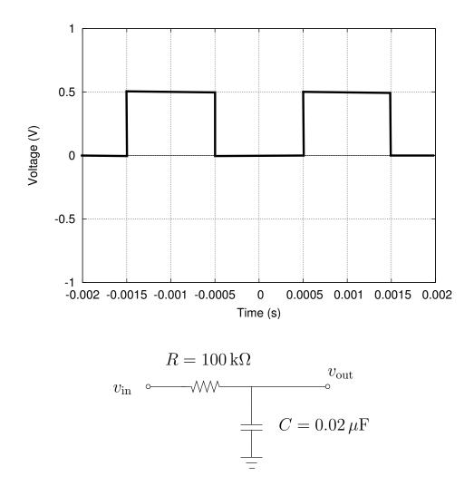
4. (20 pts) The input to the illustrated circuit is a sine-wave with angular frequency  $\omega$ . Derive a formula that gives the output voltage in terms of the input voltage and variables  $\omega$ , R, and C. Does the output lead or lag the input? (There is more than one way to do this problem.)
